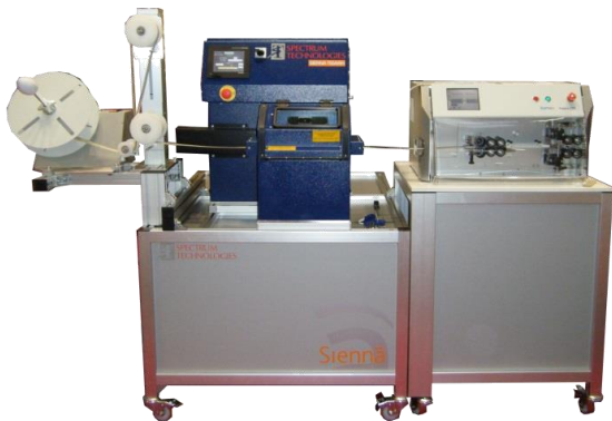
Above: A SIENNA 700 set up for automated wire handling.
